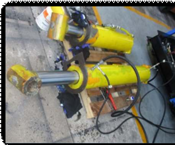
Crane Boom Cylinder Pressure Testing
