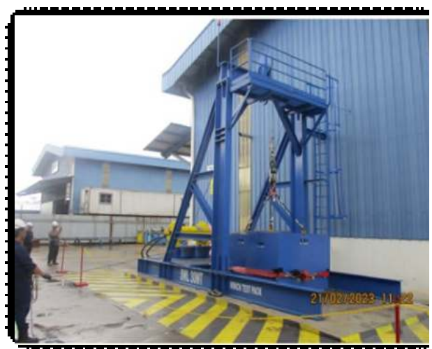
Braden Winch Load Test
